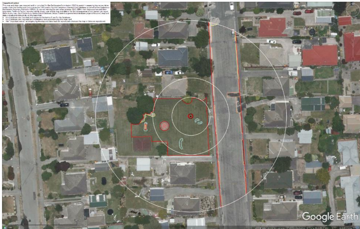
Figure 37: Aerial photograph showing the ejecta outline at the site for Dec-11 EQ.
