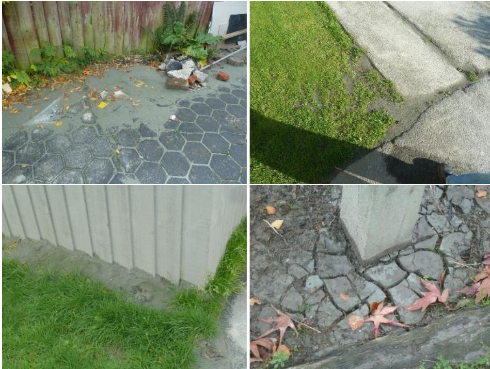
Figure 38: Ground photographs showing ejecta remnants at nearby properties (photograph date: May 2011).
